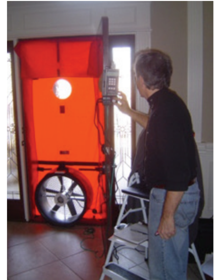
Figure 17: Blower door testing
